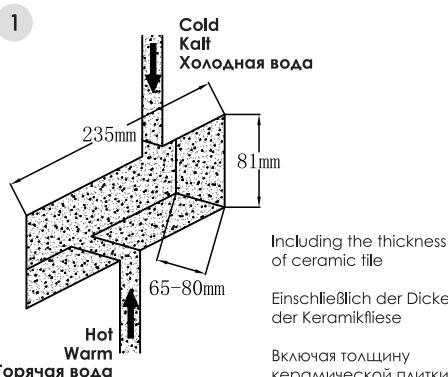
**2** Connect the hot and cold water inlet and make sure no leaking at connections.
